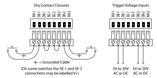
To use dry contact closures, add a jumper between the SE and DB connections, and connect the switch to other DB input and the SW input. Note that the SW-1 and SW-2 connections are also connected to the chassis ground. If you are using a shielded cable to the switch, connect the SW side to the shield. If one side of your button is grounded, the side that is grounded should use the SW connection.
