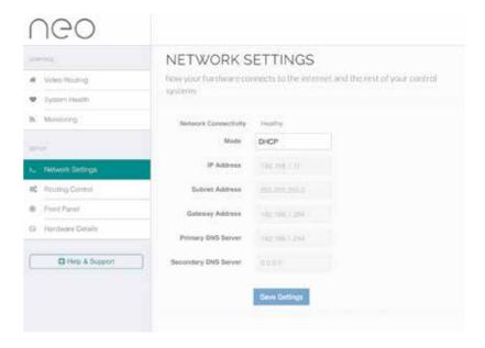
You must ensure that the new settings are correct before saving them as you will no longer be able to access the matrix if they are incorrect. In order for the internet based functions to operate such as the cloud based monitoring and gotomymatrix.com facility you must provide at least one valid DNS address. We recommend using the Google Public DNS address 8.8.8.8 for Primary DNS and 8.8.4.4 for Secondary DNS
